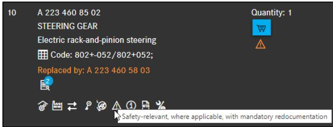
Figure 95 "Symbol for safety-relevant parts that may require redocumentation"
