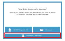
After restarting your computer, this Hardware Selection Window will open. Please select "Simulation without VCI". Then, the ConfigAssist Tool will open automatically.
